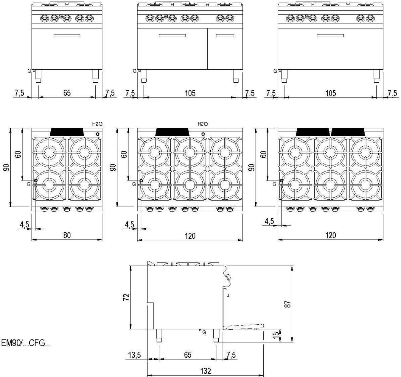
MISURE IN cm - DIMENSIONS IN cm - ABMESSUNGEN IN cm - MESURES EN cm - MEDIDAS EN cm - MATER IN cm
