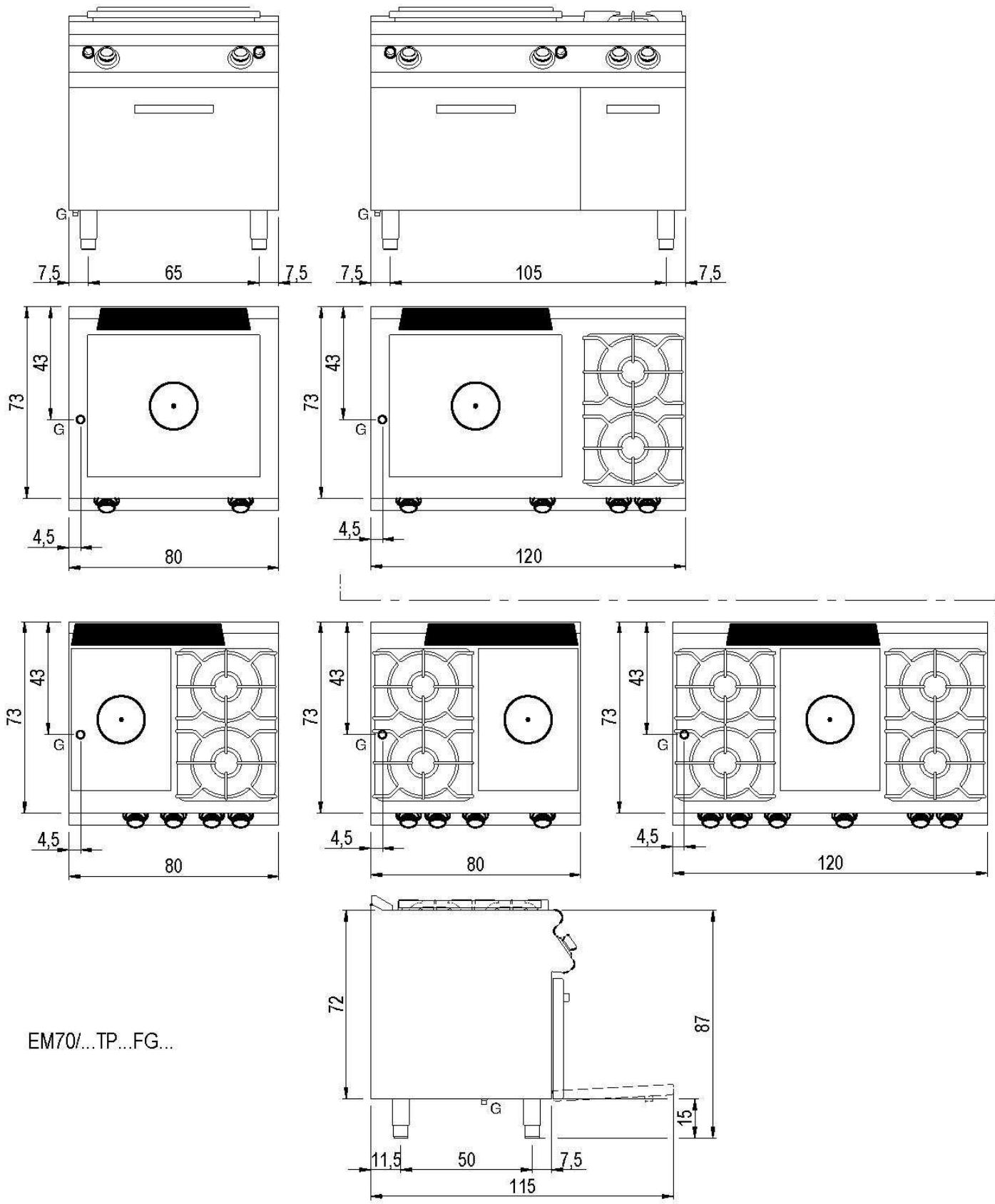
MISURE IN cm - DIMENSIONS IN cm - ABMESSUNGEN IN cm - MESURES EN cm - MEDIDAS EN cm - MÄTEN IN cm
