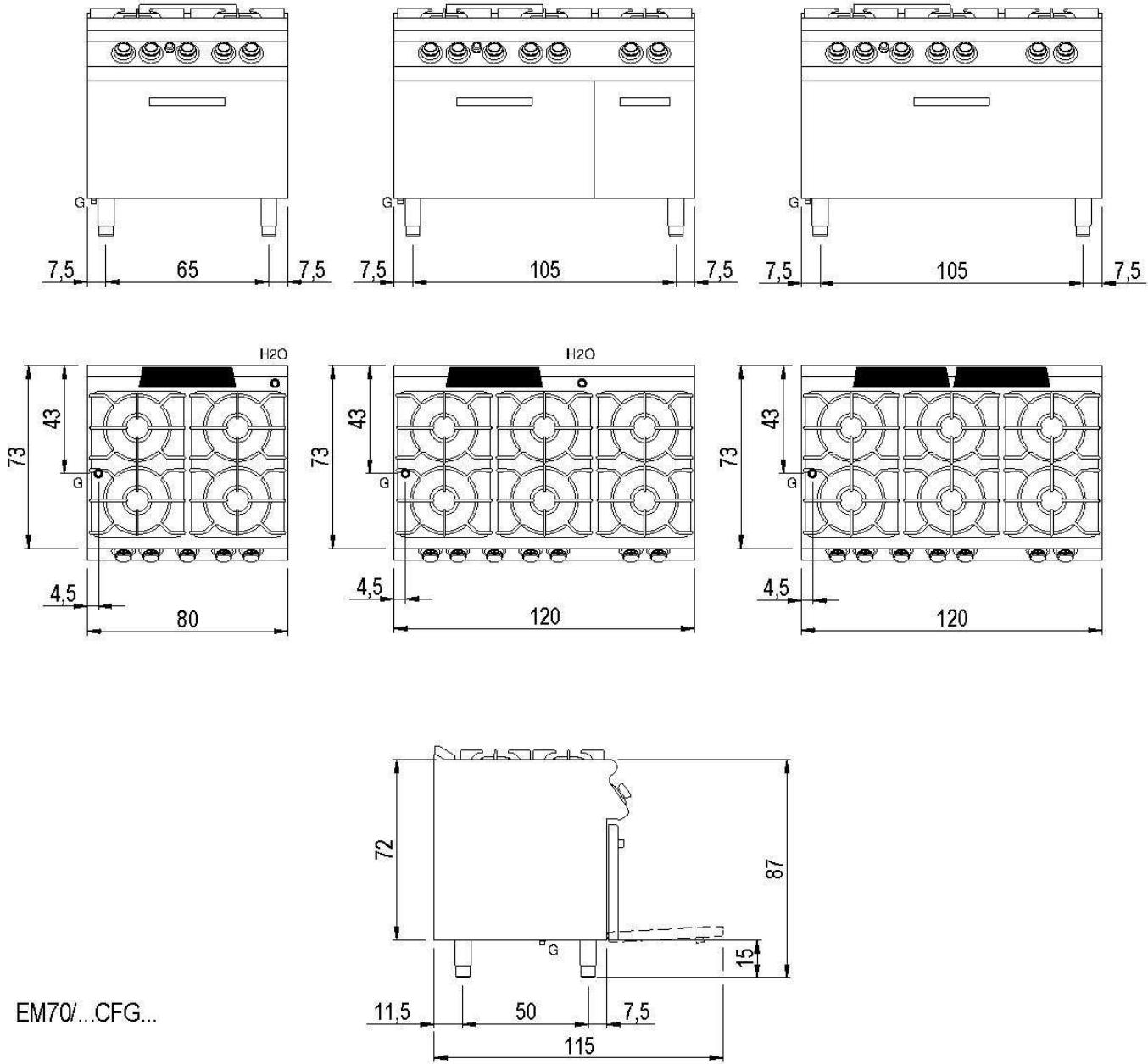
MISURE IN cm - DIMENSIONS IN cm - ABMESSUNGEN IN cm - MESURES EN cm - MEDIDAS EN cm - MATEN IN cm
